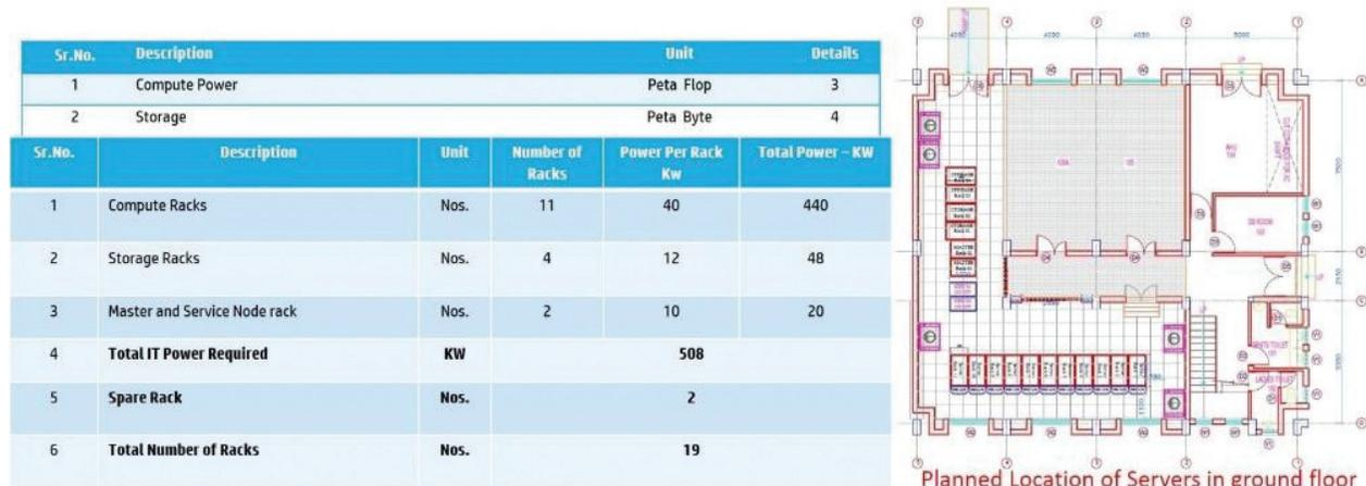
**Figure. IUAC Computing facility specification with physical lay out**
