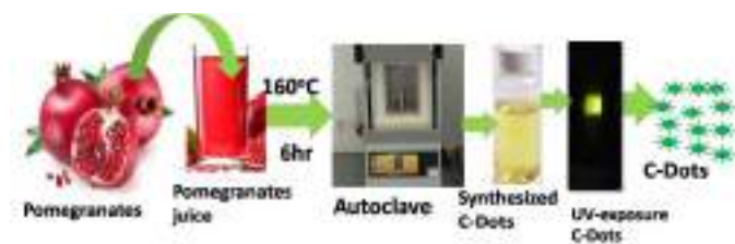
Fig.1. Schematic illustration for the hydrothermal synthesis of c-dots from Pomegranates juice having green photoluminescence.
