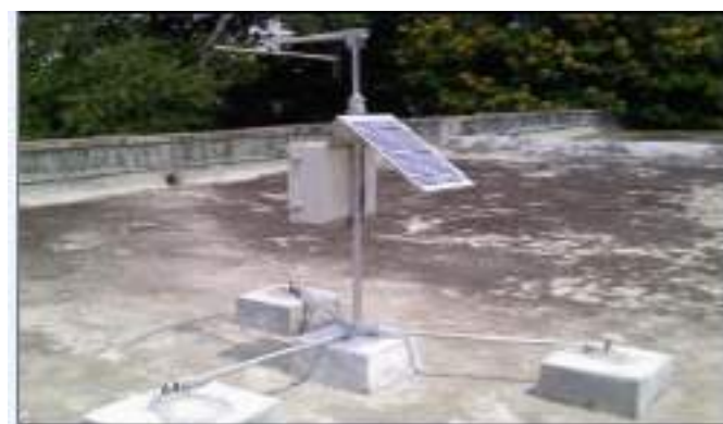
Fig.2: Digital Solar Radiation Pyranometer in EE dept. of VNIT Campus.
